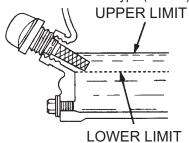
Figure 6. Engine Oil Dipstick
